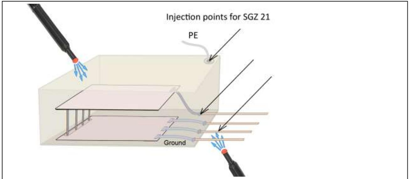
Figure 20: Complete device with housing and printed circuit boards.
