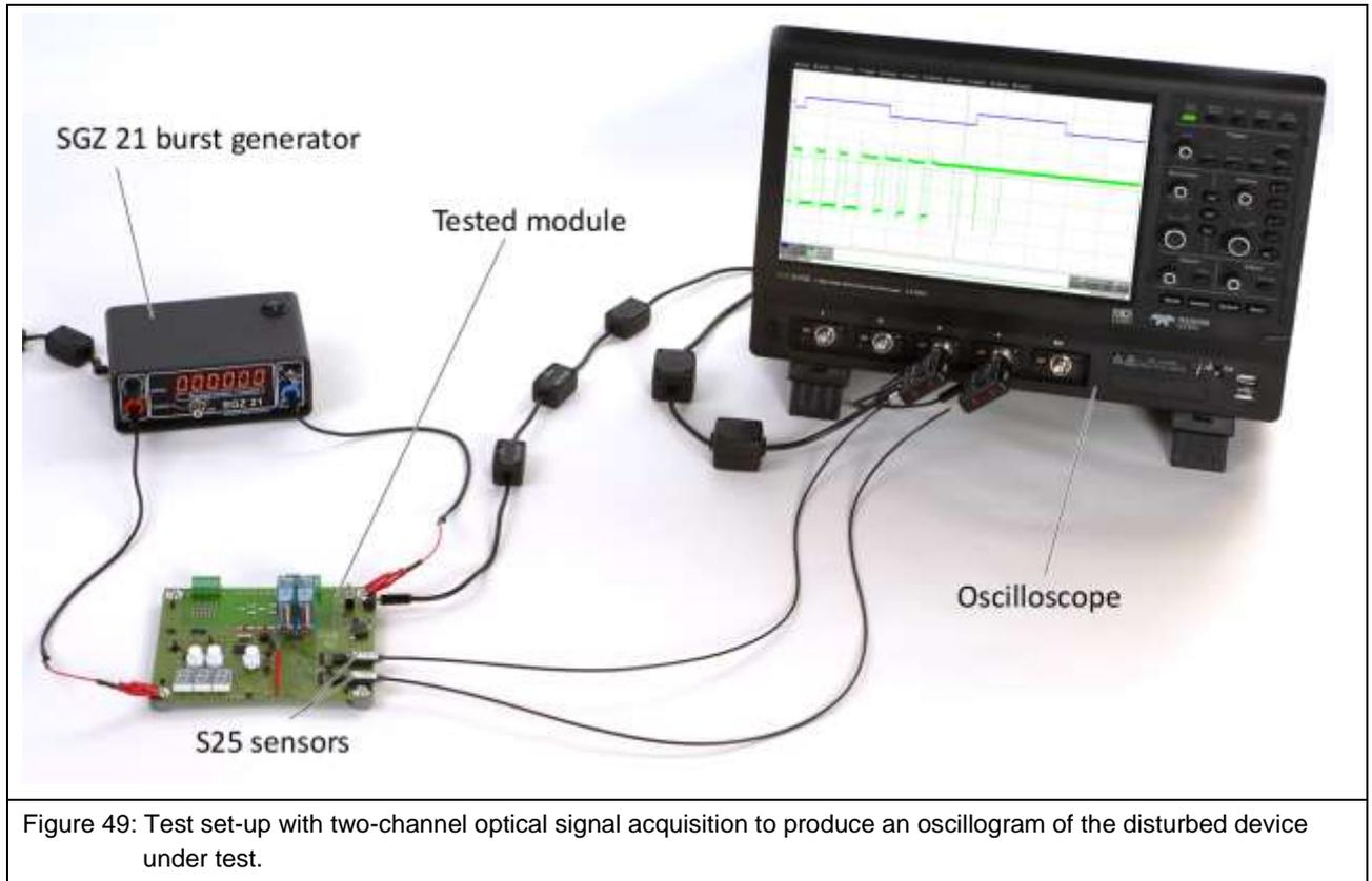
Figure 49: Test set-up with two-channel optical signal acquisition to produce an oscillogram of the disturbed device under test.
