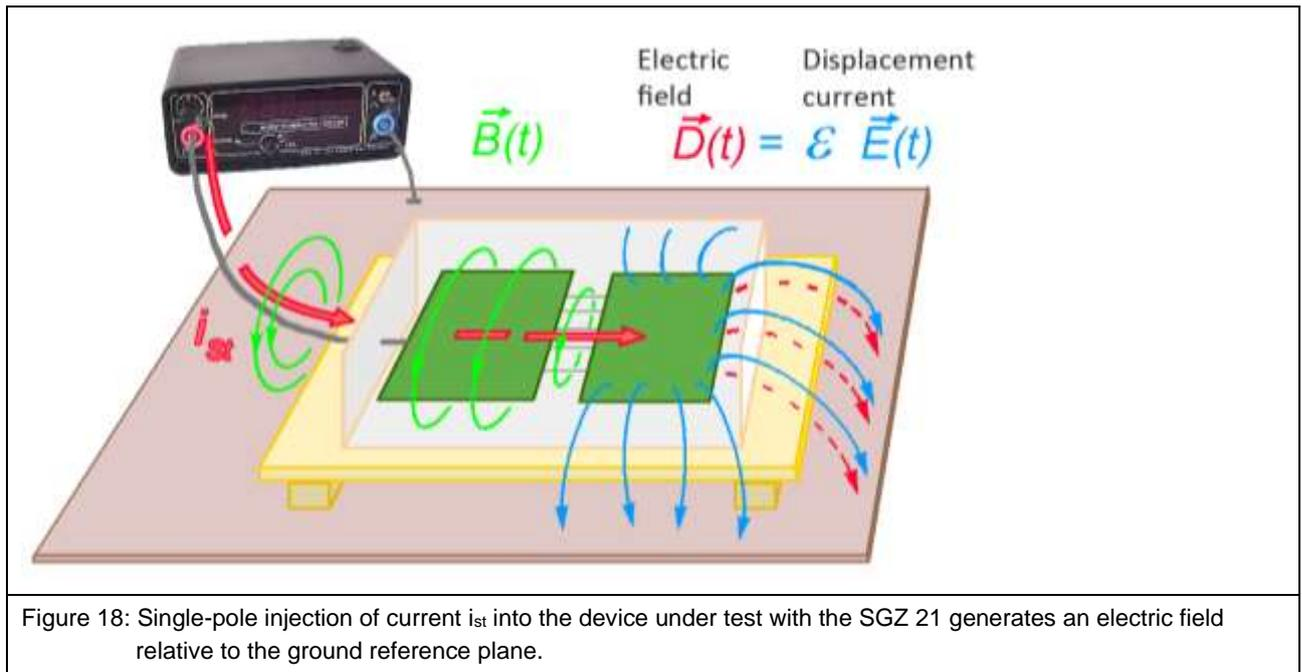
Figure 18: Single-pole injection of current  $i_{st}$  into the device under test with the SGZ 21 generates an electric field relative to the ground reference plane.
