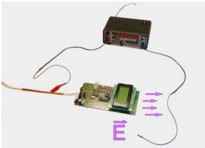
Figure 29: Single-pole injection of the disturbance current with the SGZ 21 burst generator generates an electric field to the generator's counter-pole.
