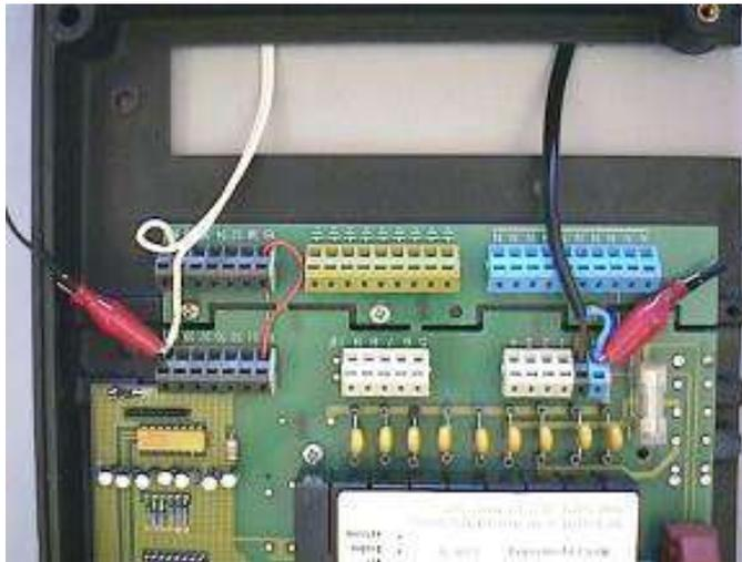
Figure 24: Injection of disturbance current into the device under test via a two-pole connection and a galvanic isolating point.
