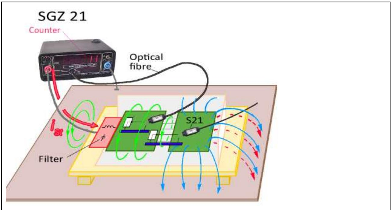
Figure 44: Dimensioning of filters with the pulse density method.
