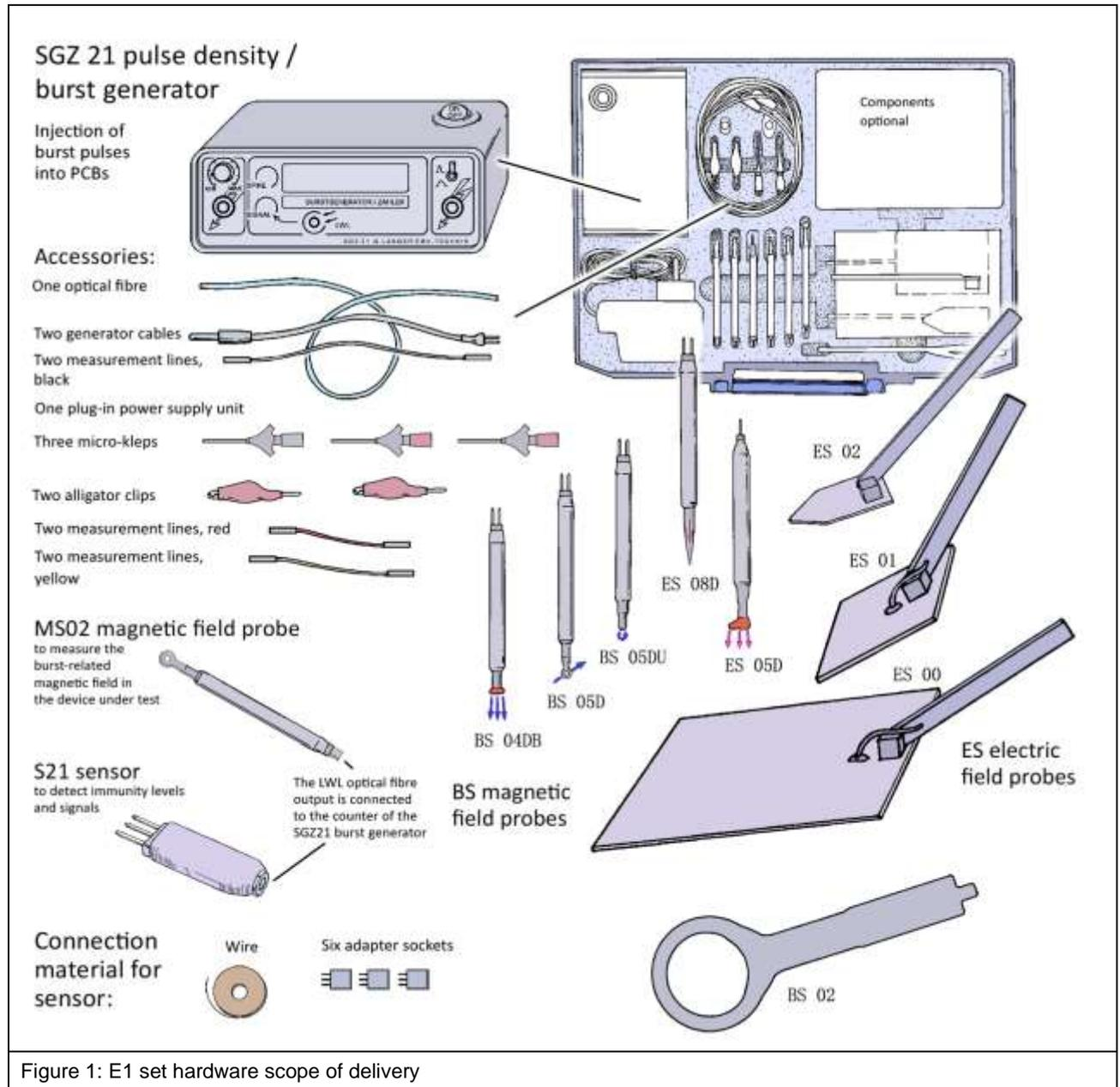
Figure 1: E1 set hardware scope of delivery
