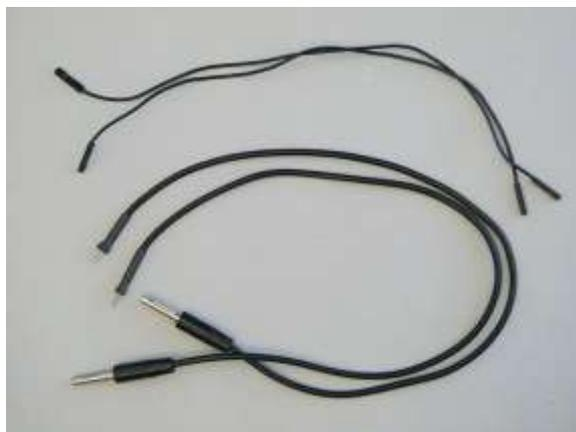
Figure 3: Generator cables (bottom); two extension cables (top).
