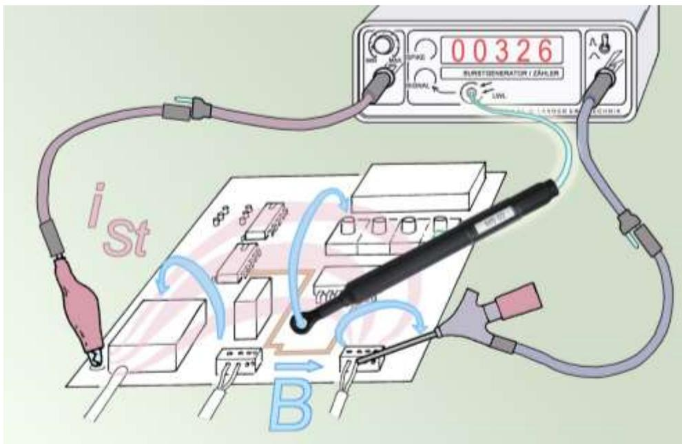
Figure 46: Operational principle of the MS 02 magnetic field probe in connection with the SGZ 21.
