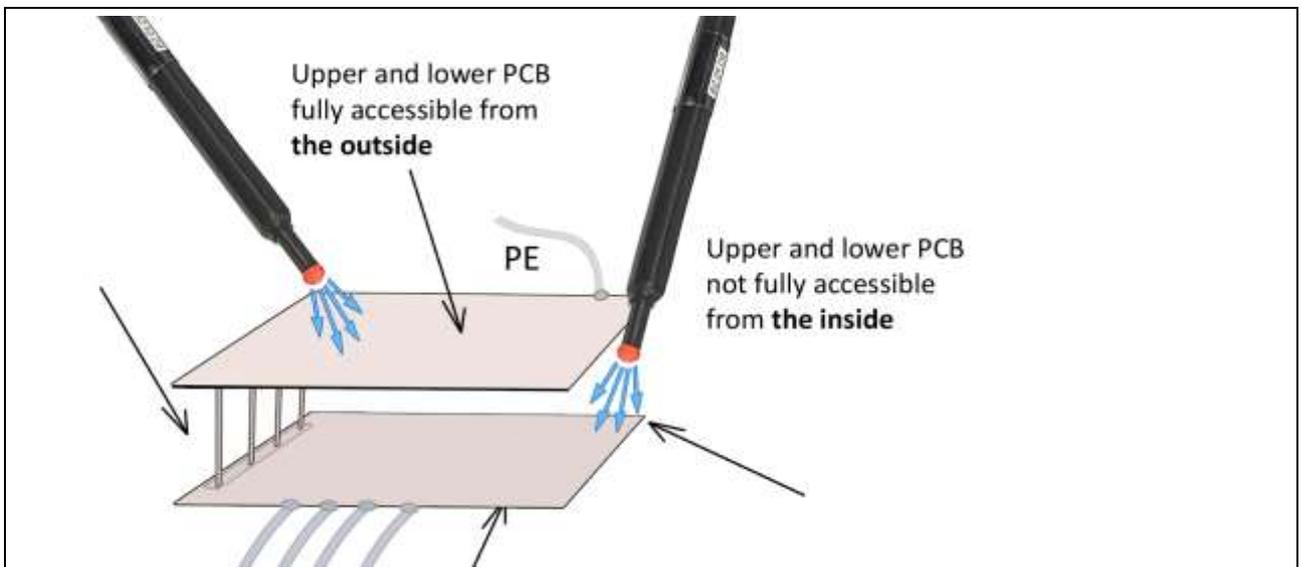
Figure 21: Device without housing; the printed circuit boards are connected and functional.
