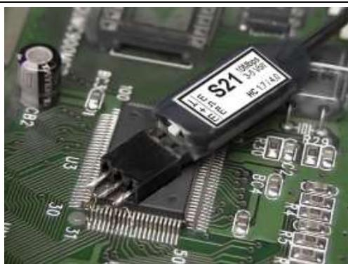
Figure 9: S21 sensor connected to an IC in the device under test, for example, via a three-pole socket.
