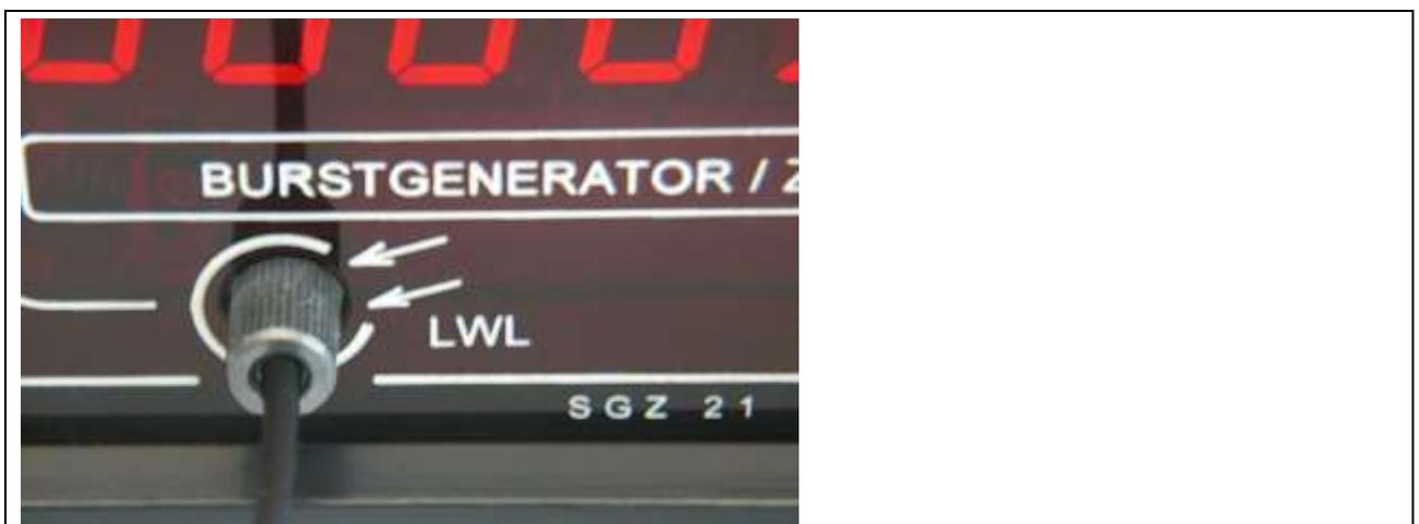
Figure 6: Optical fibre connection on the SGZ 21.
