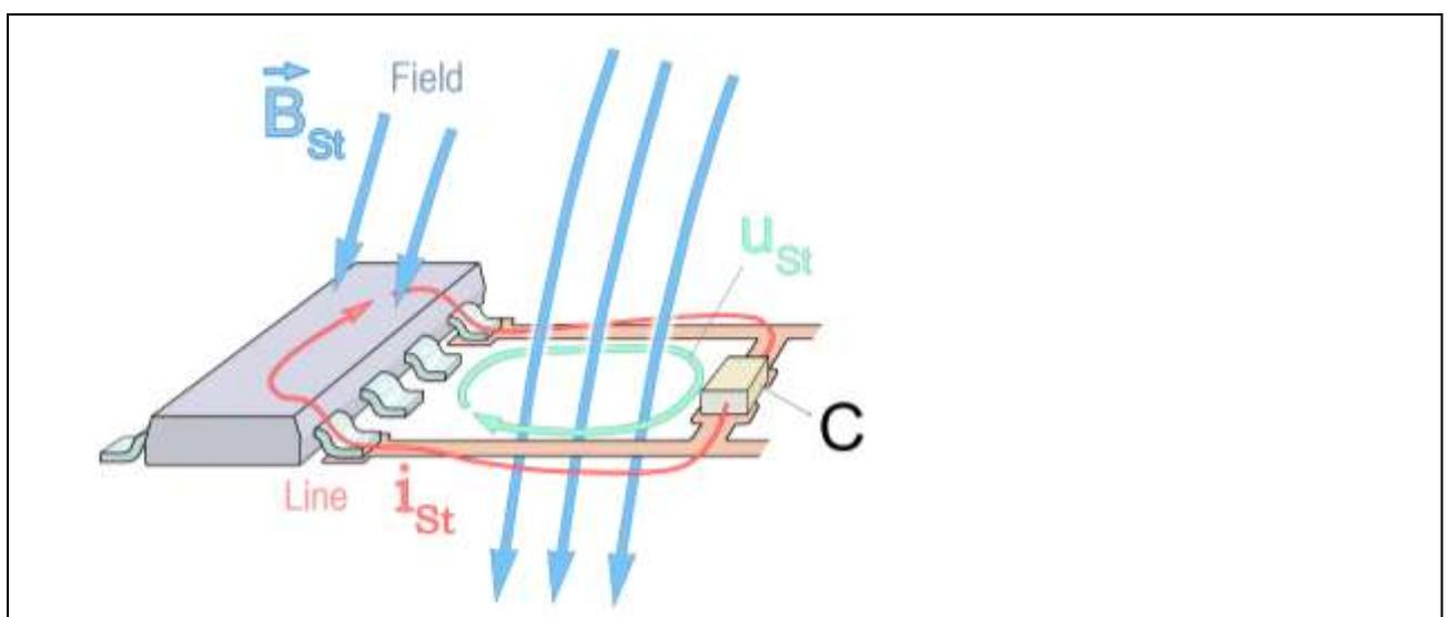
Figure 32: Principle of magnetic coupling to conductor loops.
