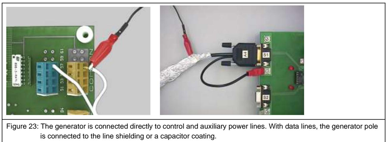
If the disturbance current is injected via a printed circuit board, the generator poles are connected to the board's ground at existing ground points such as terminals, component connections, etc. (Figure 24). If the printed circuit board has a galvanic isolating point, this can be used for injection (Figure 24).
