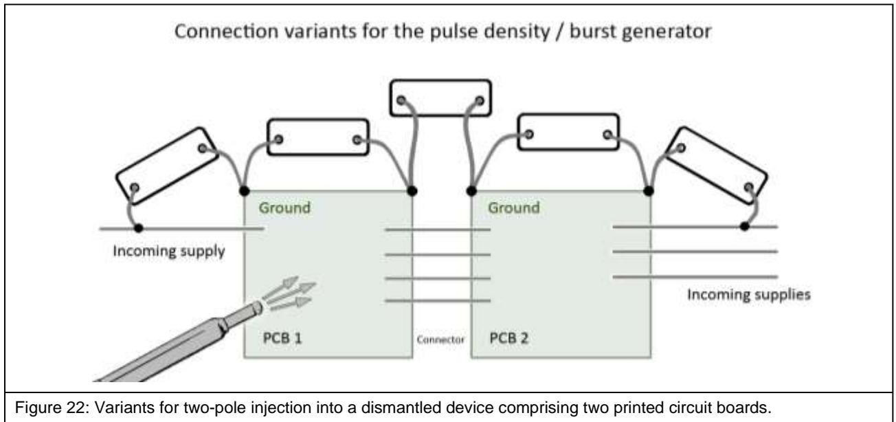
The printed circuit boards of the device under test are now fully accessible and disturbance current can be selectively coupled to them via a two-pole connection.
