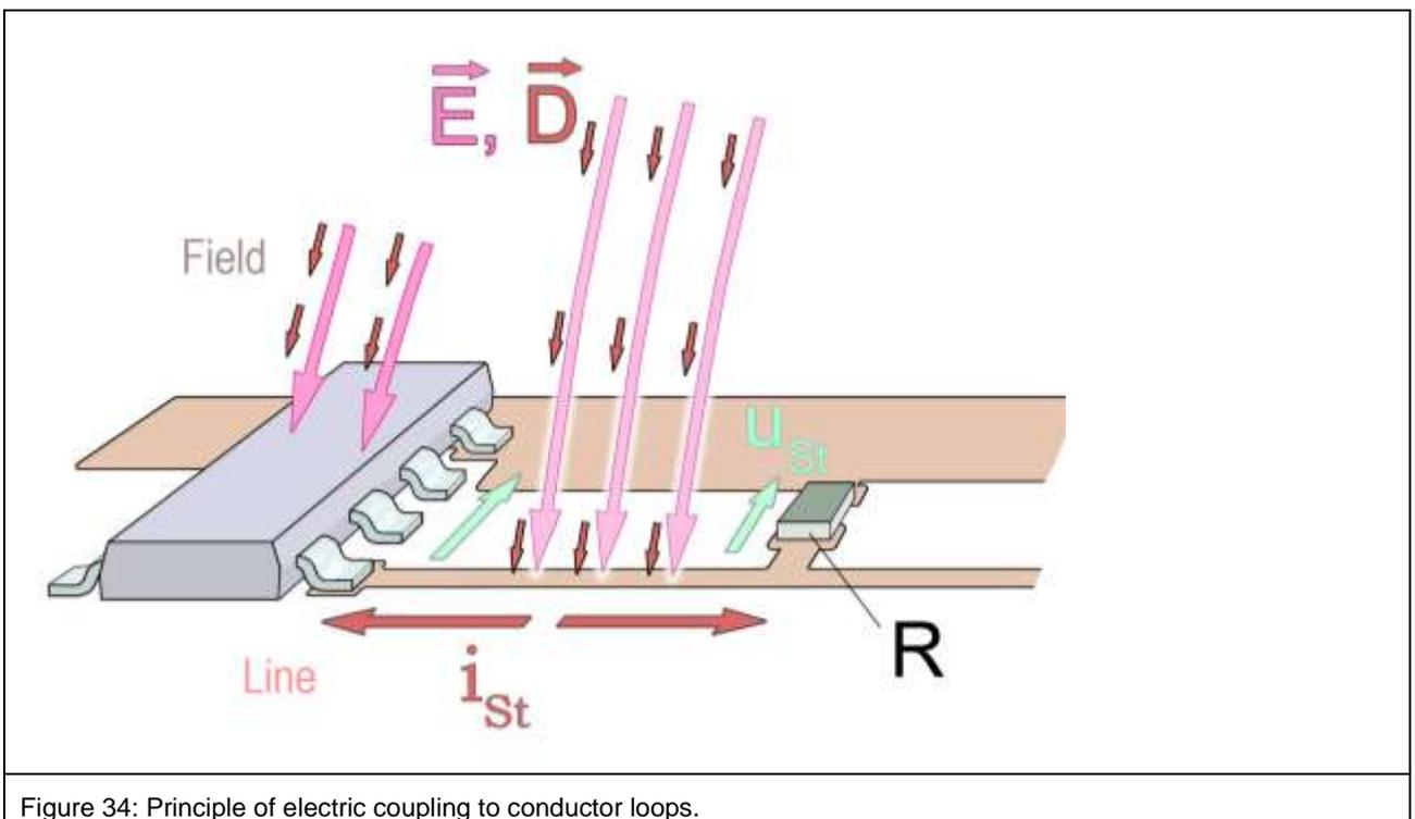
Figure 34: Principle of electric coupling to conductor loops.
